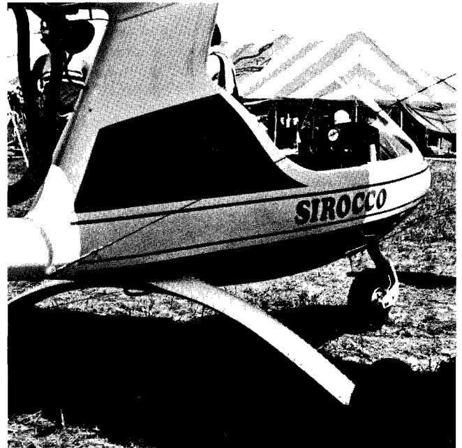
Unique hollow landing gear leg shows well in this picture. Note very smooth finish on fuselage.
