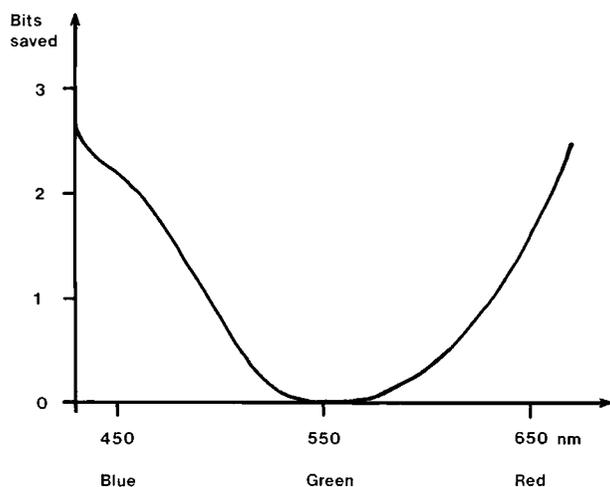
FIG. 3. Possible bit savings for image display as a function of wavelength.
