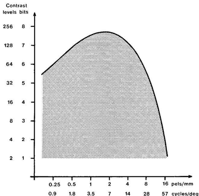
FIG. 1. Contrast sensitivity of the visual system, as a function of spatial resolution (after Robson<sup>10</sup> and Mannos and Sakrison<sup>8</sup>).
